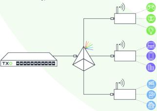
In the infographic above you'll see that an Optical Line Terminal (OLT) sends a single line of optical light (signal) into a splitter. The splitter contains glass elements that act as a prism to divide (or split) the optical light into multiple identical waves of signals down individual fibres which are connected to an Optical Network Unit (ONU). This is a termination point where the end-user can leverage the signal for work, home and leisure activities.
